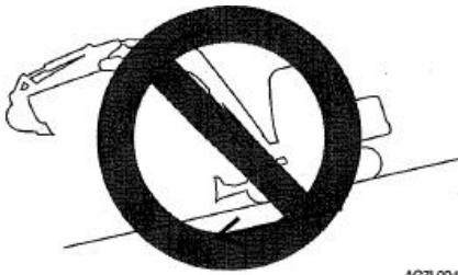
Steep slope when the attachment is lifted
